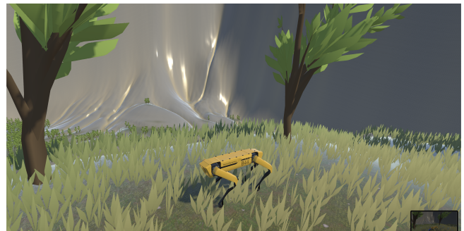
Figure 1: A to-scale Spot robot as viewed via the Meta Quest 3. The robot traverses the simulated environment, enabling testing of our algorithm for robot trajectory optimization in a robust and realistic environment.
