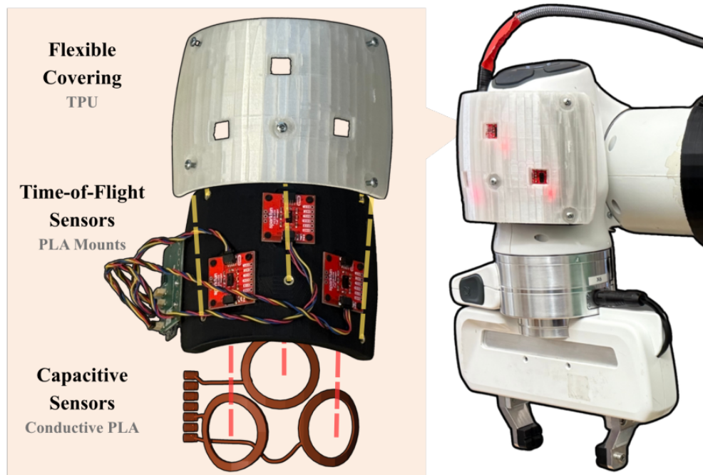
Figure 2.2: The hybrid sensors are composed of three layers: 1) self-capacitance sensors, 2) ToF sensor mounts, and 3) compliant soft covering.
