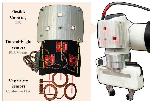
Fig. 1: The hybrid sensors are composed of three layers: 1) SC sensors, 2) ToF sensor mounts, and 3) compliant soft covering.
